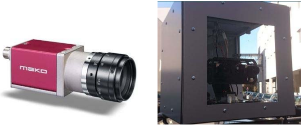
Fig. 4. Camera MAKO Gigabit Ethernet and Acquisition support.
